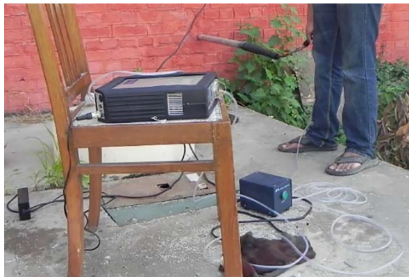
Fig. 1 AVL 244 di-gas analyzer for detection of emission from algal biodiesel–petro-diesel blends
